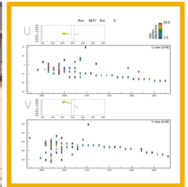
A picture of a typical interaction of a muon-flavor neutrino. The muon produced in the interaction (the long track in the picture) is gradually losing energy as it goes through the steel plates. The magnetic field present in the steel causes the muon to bend. The amount of bending gives a measurement of the muon energy.
