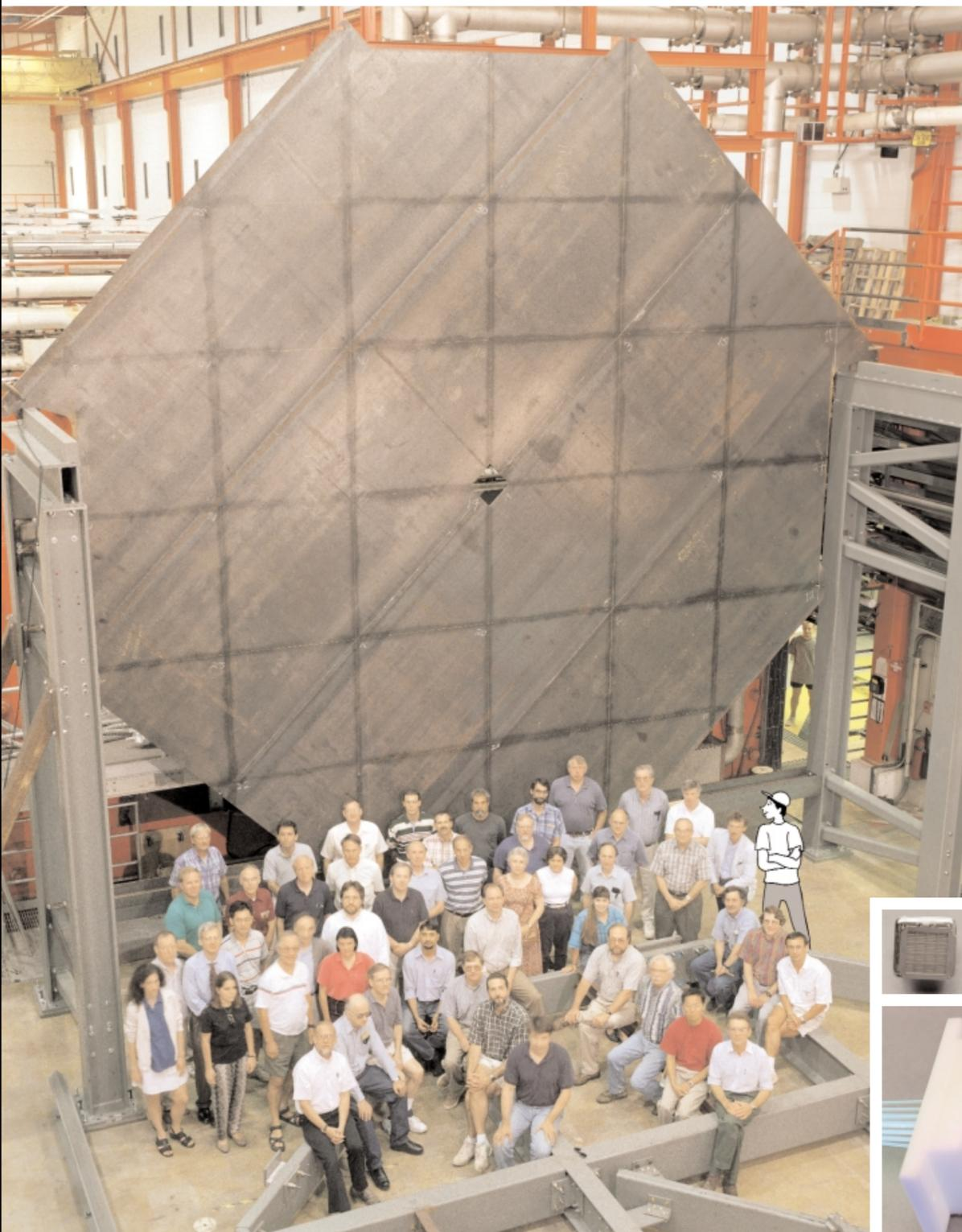
The MINOS collaboration poses for a photo in front of a steel plane of the MINOS detector. Eventually the detector will be 90 feet long and 24 feet in diameter, made of 486 layers of these eight-sided steel plates. Even with 5,000 tons of steel, only a few in 10 billion neutrinos coming from Fermilab will interact in the MINOS detector.
