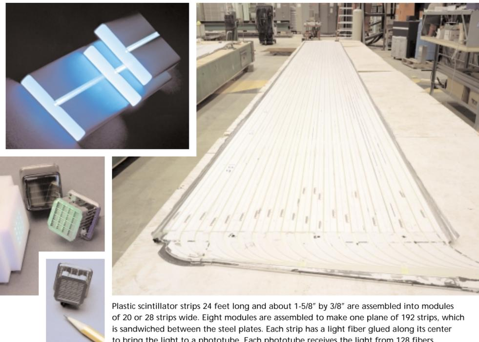
Plastic scintillator strips 24 feet long and about 1-5/8" by 3/8" are assembled into modules of 20 or 28 strips wide. Eight modules are assembled to make one plane of 192 strips, which is sandwiched between the steel plates. Each strip has a light fiber glued along its center to bring the light to a phototube. Each phototube receives the light from 128 fibers.
